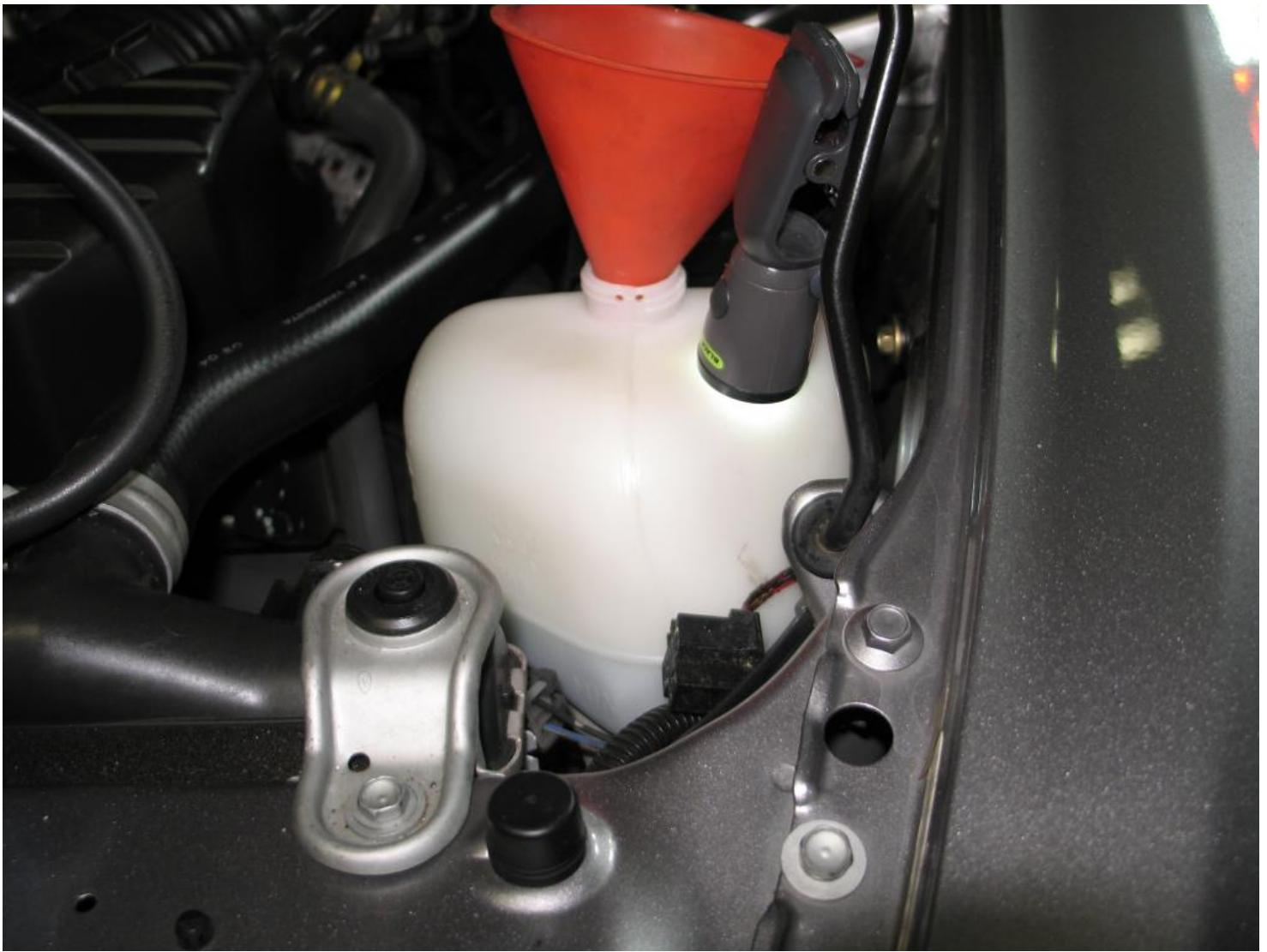
Now its time to fill the rad. Pay attention here. Expect to fill it with 6.5 to 6.6 litres. I kept track (i actually measured it) of how much coolant came out so expect the same amount to go back in.
