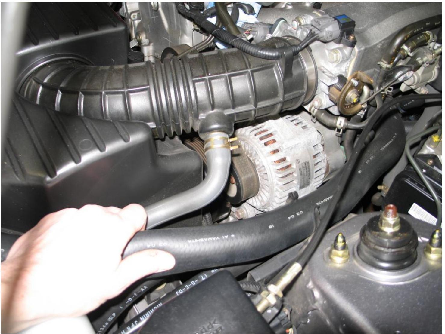
OPEN BLEEDER. ADD COOLANT. SQUEEZE...till more coolant comes out the front air bleed. CLOSE THE AIR BLEED. More coolant into the rad- unless the rad is overflowing.
