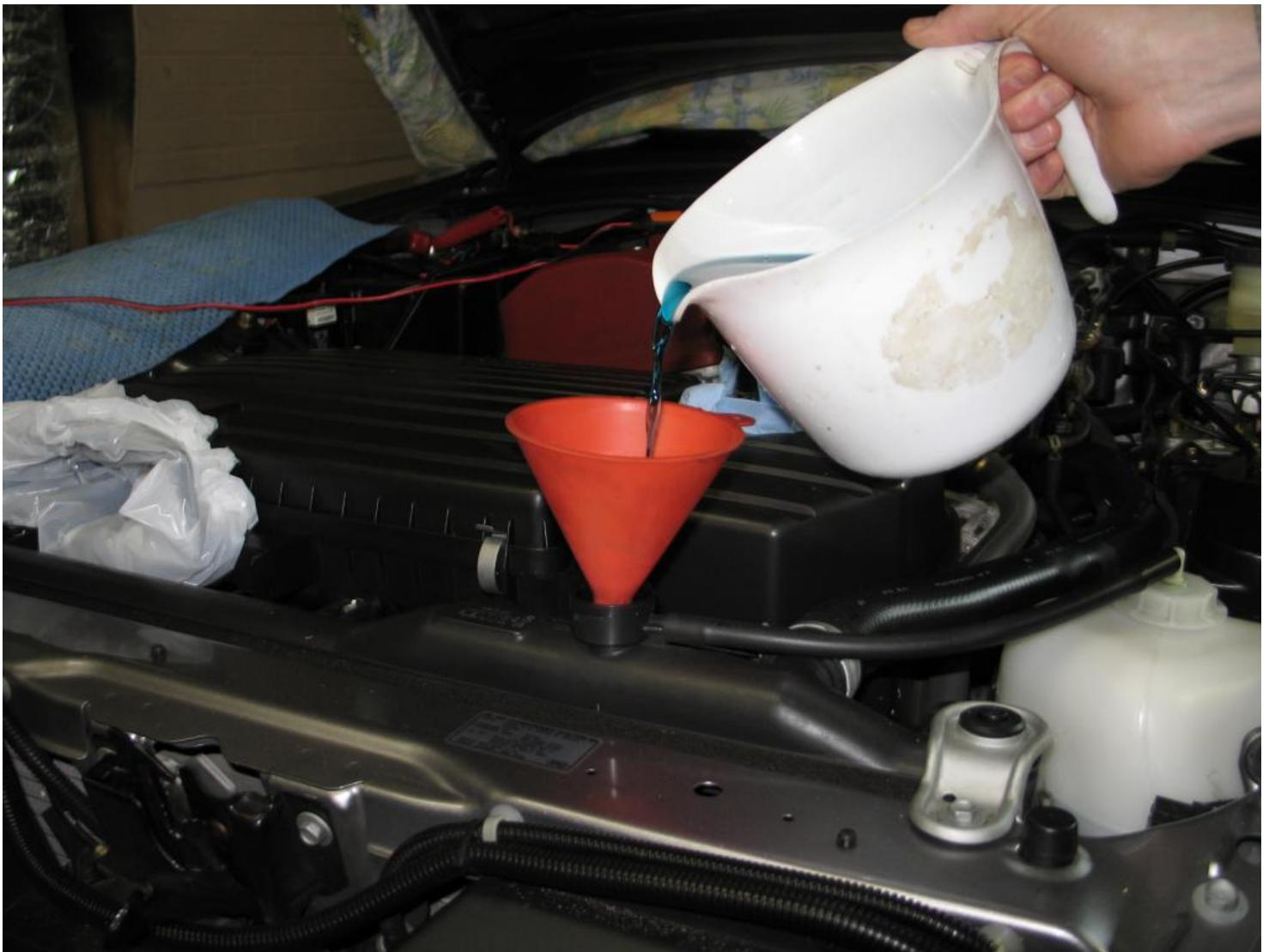
I used a 1400 ml container to keep track. Keep filling until coolant comes out of the FRONT AIR BLEED BOLT. NOW CLOSE IT. Squeeze the top rad hose to flush coolant around more. You can even seal your hand over the rad fill while you squeeze to force more of the coolant around. Just remember that the Front air bleed bolt allows that pesky air to bleed out- obvious, eh?
